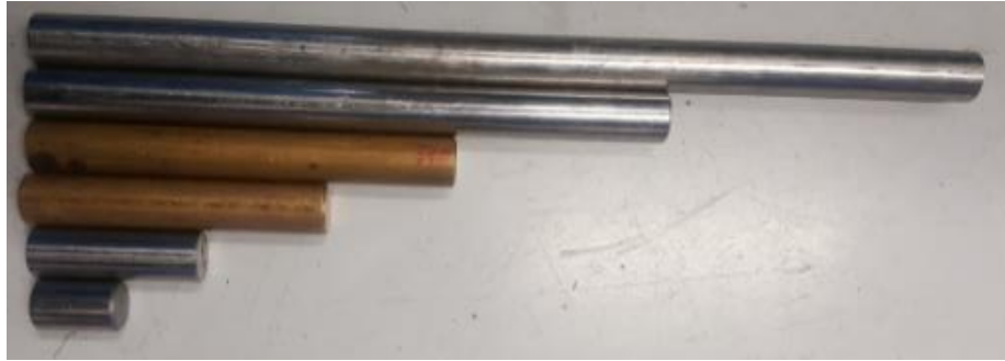
Figure 3.17 - Cylindrical projectiles with masses 250g, 500g, 1000g, 1500g, 2000g, 3000g (bottom to top).
