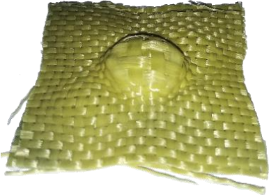
Figure 4.1 - Plain-woven aramid after impact test.
