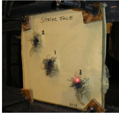
Figure 2.19 - Example of experimental test on a ballistic panel with 3 impact zones [Nayak, 2016].
