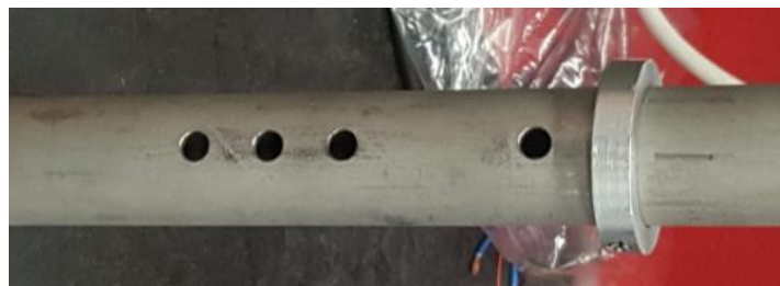
Figure 3.15 - Illustration of tube with holes for air outlet.
